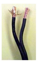
Although this cable is double-screened with copper braid on copper foil, it is not as efficient as, say, H109 and should not be used in lengths greater than 20 metres. Nor should it be joined at any point. A straight run without "discontinuities" is essential.
