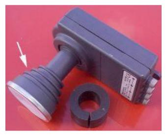
If it is incorrect then horizontally- and vertically polarised signals will interfere with each other, resulting in loss of "quality" - "blocking" or "pixellisation" or "picture freezing" and complete loss of picture and sound on some channels. Another view of the Sky-plus Quad-output LNB, showing the Here is a standard Quad-output LNB. Notice the circular scalar rings of the feed horn.
