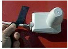
50mm away from the "F" connector. Stretching the tape, wind it around the cable with an overlap of half the tape width until the tape touches the LNB body. Continue stretching and winding until you get back to the starting point. Cut the tape from the reel at this point. The "F" connector should be covered completely by the tape which will have welded itself to form a tight rubber tube.
